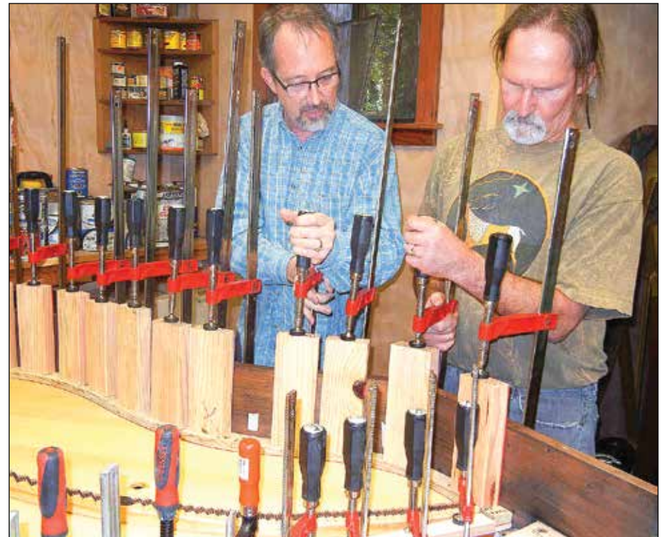
FINE-TUNING — Dave Hankin, right, and Humboldt State University piano technician Greg Granoff go through the precise and laborious process of installing a new sound board in a 1920 Mason & Hamlin grand piano. Submitted photo.
